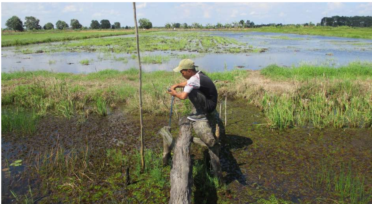
Gambar : Pengukuran kecepatan arus air disaluran lahan pertanian Desa Terusan Karya. / Measuring the water flow speed in farmland channel of Terusan Karya Village.
