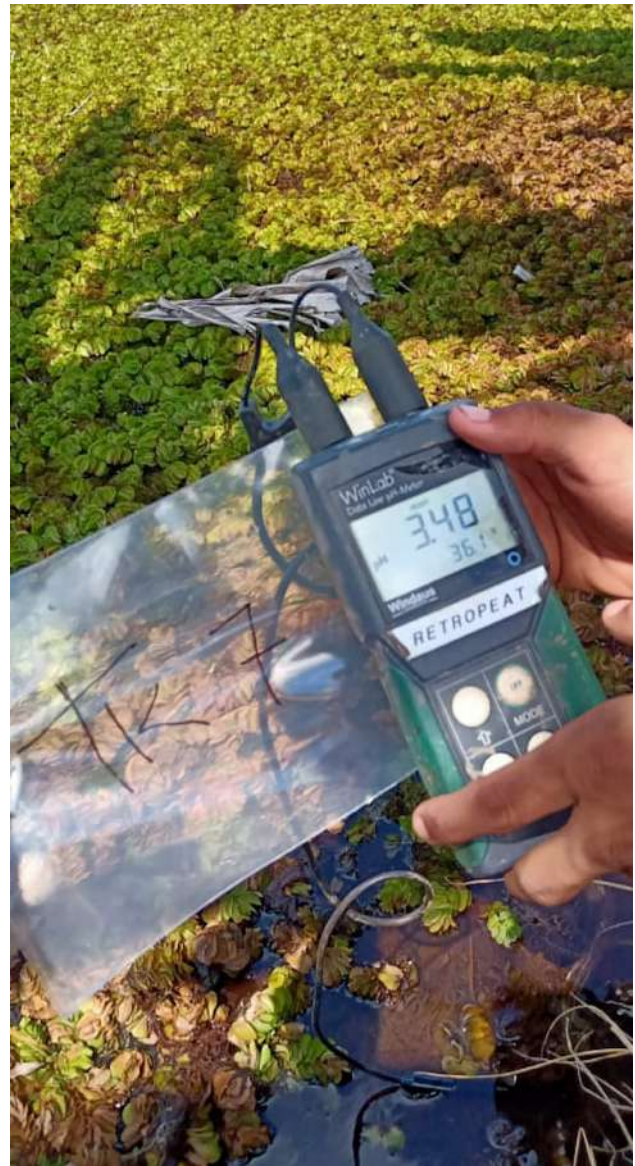
Gambar : Alat PH meter menunjukkan kadar PH rendah atau asam di saluran pertanian Desa Terusan Karya. / PH meter tool showed low PH or acidic concentration in farming channel in Terusan Karya Village.
